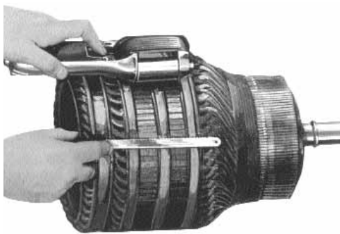
Type U-2 Universal Adjustable Growler may be used as both an external Growler for armatures and an Internal Growler for stators.
